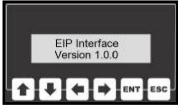
The human-machine interface or HMI consists of an 2-line by 16 character backlit LCD display and a six-button keypad. During power-up, the display on the HMI will display the firmware version contained inside the microprocessor's memory.
