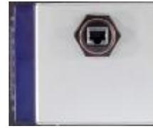
The Ethernet port is used to transmit and receive TCP/IP messages that are formatted to comply with Ethernet IP.
